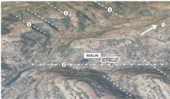
Figure 3: Oblique view of Google 3D image with representatively shown E-W fracture swarms (1) and ENE-WSW fracture valley (2), Malin Area.
